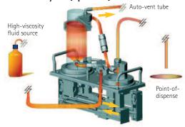
Air is vented from the topmost point of the filter housing, through the vent valve.
