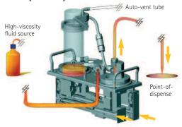
Precise volume of chemical is dispensed onto the wafer at a user-programmable, controlled rate.
