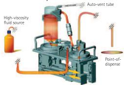
Chemical is filtered at a slower rate than the dispense rate.
