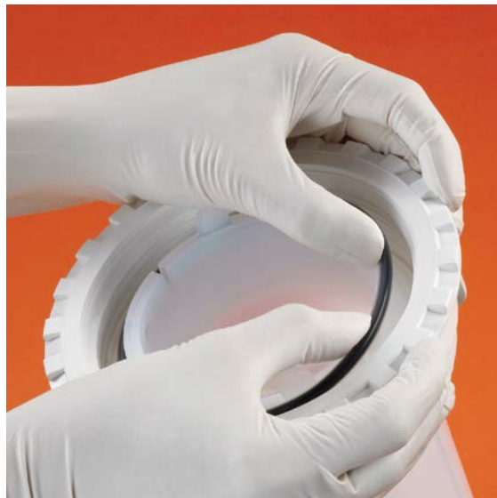
Installation of the o-ring onto the Chemlock housing using clean gloves to minimize possibility of contamination.
