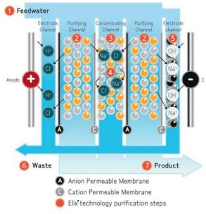
Merck Millipore's Elix® module: unique technology based on anion-permeable and cationpermeable membranes; high-quality ion-exchange resin; and activated carbon beads.
