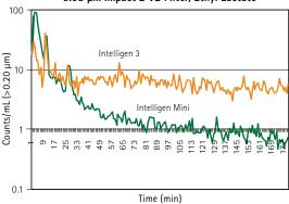
In side-by-side testing with the IntelliGen 3 dispense system, the IntelliGen Mini dispense system demonstrated both rapid priming and an order of magnitude reduction in liquid particle counts.
