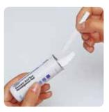
Remove one  $MQuant^{TM}$  test strip from the protective tube.
