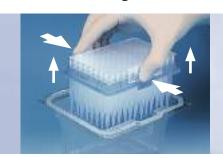
Press the long sides of the transfer aid together, and continue pressing them together while withdrawing the tip-tray.
