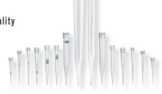
For the manufacture of pipette tips and filter tips, BRAND exclusively uses raw materials that are free from the additives di(2-hydroxyethyl)methyldodecylammonium (DiHEMDA) and 9-octadecenamide (oleamide). Both of these additives are frequently found in PP granules, and can interfere with biological tests, leading to spurious results. Only highly polished tooling equipment is used, so that no parting agents or demolding aids are needed.
